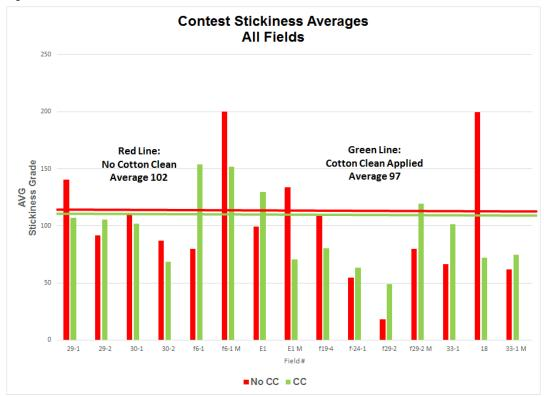
However, when fields with lower levels of stickiness (<100 stickiness grade) were removed from the averaging process, the result is dramatically different. When only those fields with medium to heavy stickiness were considered, Cotton Clean™ applied at ginning reduced measured stickiness significantly, from 147 down to 97, a reduction of 34%. See CHART 2.
